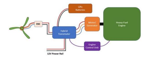
The hybrid architecture of the system allows for bidirectional power flow between the electrical system and the engine.
