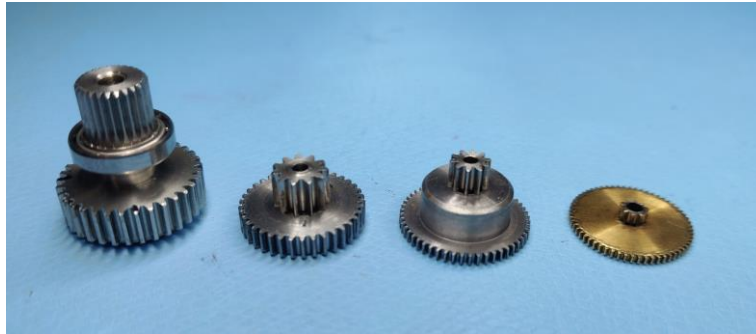
Figure 8- Servo gears, cleaned after the test ready for inspection. Gears referenced as 1 to 4, left to right.
