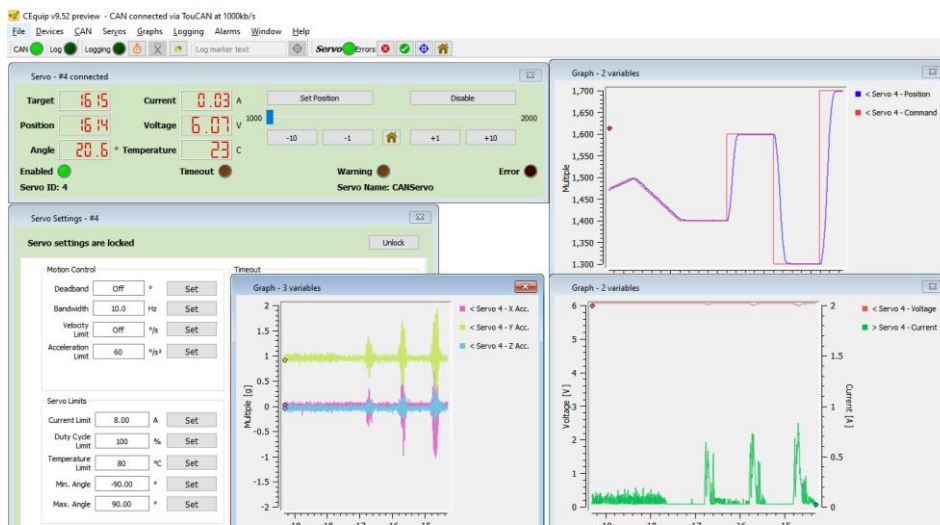
Figure 2: CEquip software showing: servo status, servo settings and graphs of actual position, commanded position, current, voltage and accelerometer data.
