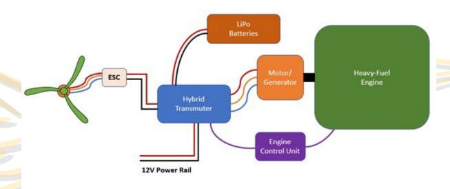
The hybrid architecture of the system allows for bidirectional power flow between the electrical system and the engine.
